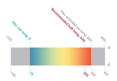
Eastman Marlotherm<sup>®</sup> SH heat transfer fluid is a synthetic heat transfer fluid that offers outstanding performance during both lowtemperature start-up and high-temperature operation. It performs over the entire temperature range without being kept under pressure. When operating in a well-maintained heat transfer system, Marlotherm SH provides reliable, consistent performance over long periods of time.
